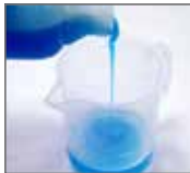
Add bi-component gel in a 1:1 ratio
