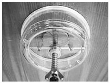
5. Cut hole by attaching a power drill to the top of the cutter.
