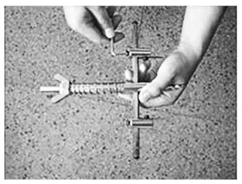
1. Adjust the distance between the two blades to match the required hole size to be cut.
