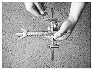
1. Adjust the distance between the two blades to match the required hole size to be cut.
