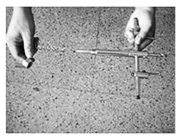
2. Unlock and remove the spring and nut from the hole cutter.
