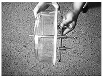
3. Insert the cutter into the transparent cover.
