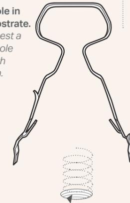
Slide the clip over the cable. Make sure it's seated in the rounded area of the clip.
