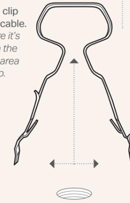
Compress and push it home. Pinch the legs together and push into the hole by hand.
