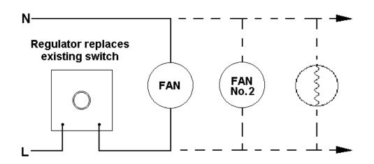
Reconnect the wires either way round to the "C" terminal and the "L1" terminal.
