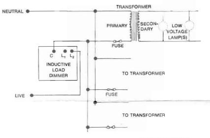
Push on/push off dimmers have three terminals. For 1-way circuits, connect wires either way round, to C and  $L_2$ . Push on/push off dimmers can be used in 2-way lighting circuits where the two switched lives should be connected to  $L_1$  and  $L_2$ . If in doubt, consult a qualified electrician.
