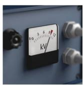
Our screwdrivers are tested for dielectric strength under a 10,000 volt load to make sure that their most important property, their insulation, has been exhaustively tested. Each individual Wera VDE screwdriver is subjected to this test to guarantee safe working up
