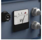
Each Kraftform Kompakt VDE set has been tested individually at 10,000 volts, in accordance with IEC 60900.This ten-times-higher testing load guarantees safe working at their maximum permitted load of 1,000 volts. Handle/interchangeable blade system
