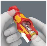
The Turbo function can either be switched on or off by pressing a button. For initial loosening and final tightening at increasing torque moments (or fine torque adjustment) of screws the Turbo function is disabled. For free running screws the Turbo function is enabled.
