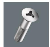
TRI-WING® The screwdriving system is mainly found in aviation and household technology (here e.g. on live components). The asymmetric arrangement of the three profile flanks prevents the use of anything other than the original tools. The high-precision Wera profile design ensures a secure fit of the tool in the head of the screw. The blades are manufactured out of bit material. The Wera know-how with regard to the hardening technology ensures a long service life of the tool.
