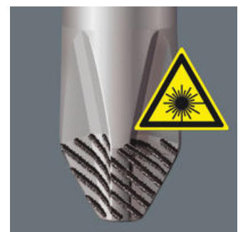
A precisely-focused laser creates a sharp-edged surface structure. This laser treatment results in an edge hardness of up to 1000 HV 0.3. Wera Lasertip "bites" itself into the screw head and prevents any slips out of the recess. It is available for screwdrivers for slotted, Phillips and Pozidriv screws.
