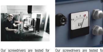
Our screwdrivers are tested for dielectric strength under a 10,000 volt load to make sure that their most important property, their insulation, has been exhaustively tested. Each individual Wera VDE screwdriver is subjected to this test to guarantee safe working up to 1,000 volts.
