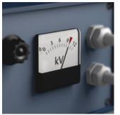
Our screwdrivers are tested for dielectric strength under a 10,000 volt load to make sure that their most important property, their insulation, has been exhaustively tested. Each individual Wera VDE screwdriver is subjected to this test to guarantee safe working up to 1,000 volts. Impact strength test
